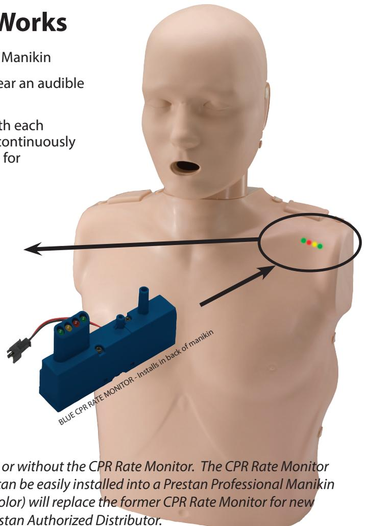
Prestan Professional Manikins may be purchased either with or without the CPR Rate Monitor. The CPR Rate Monitor is also available for separate purchase (#RPP-AMON-1) and can be easily installed into a Prestan Professional Manikin by the customer. The updated CPR Rate Monitor (new blue color) will replace the former CPR Rate Monitor for new 2016 purchases, but rollout may vary depending on your Prestan Authorized Distributor.
